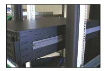
Make sure the Inner & Outer Rail match & align properly, before pushing the chassis in.
