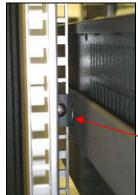
Push the release button on Inner Rail when it hits the outer rail, and again when it snaps into Outer Rail cut out, and then continue to push the chassis in (as shown in the pictures on the LEFT)
