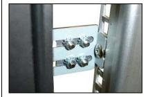
Mount the Extension brackets' slotted flange the same way as the outer rail front flange.
