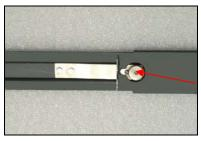
The two pictures on the LEFT show how the Inner Rail snaps into the Outer Rail and the location of the release button.
